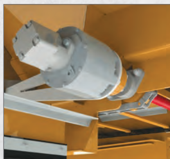
Main conveyor driven by a planetary gear, a 10 cu in motor, and a 2" drive shaft
