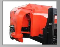
The powerful blower fan produces air velocity of 470 km/hr at the nozzles output, providing optimal cleaning performances.
