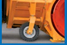
**Castor wheels** For high-speed snow removal operations, especially at airports, castors and plastic scraper blades are often used to protect surfaces.
