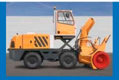
**Elevating cab** The ROLBA 600 features an (optional) elevating cab that can be variably adjusted by 700 mm in height to provide the operator with even bet-
