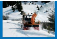
**Spot casting** Optional chutes of varied design are available for spot casting or truck loading.
